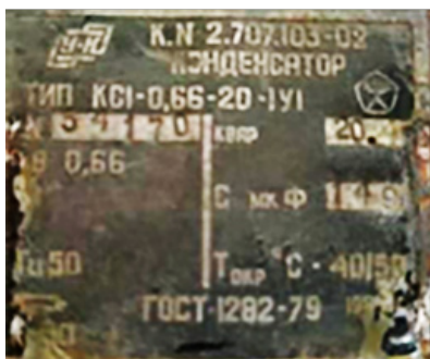
Figure: 13. Nameplates of capacitors type КС1-0,66-20-У1
